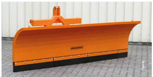
The snow blade with a working width of 2.00 m to 2.90 m is suitable for clearing paths and roads. The rubber scraper prevents damage to the road surface.
