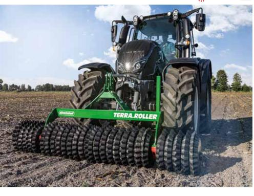
The **TERRA.ROLLER** eco with Cambridge or toothed rings is suitable for versatile tasks in arable and grassland. With the CAT 2 three-point hitch, it can be used both as a front packer as well as a three-point roller at the rear.
