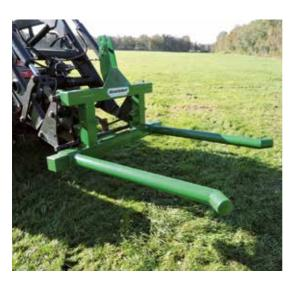
The Combi round bale fork can be used by different carrier vehicles due to its EURO and 3-point hitch.
