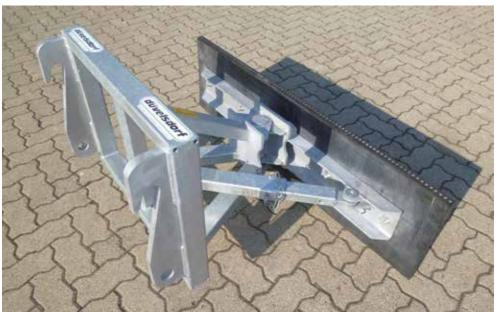
1.30 m, mechanical adjustable for Weidemann (hydraulic lock) or EURO. Hydraulic adjustment is available as an option.
