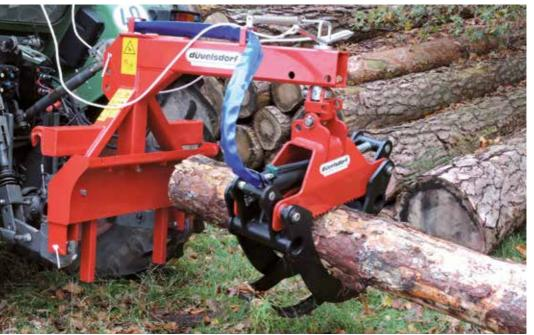
The combination log gripper has both a front loader EURO attachment and a 3-point attachment CAT 2.
