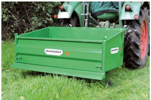
Rear containers can be used as transport containers or buckets. The standard rear container has a pendulum-mounted removable rear flap and a scrape rail.
