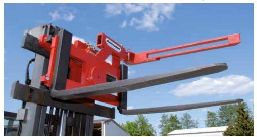
The düvelsdorf crate rotating devices fit all forklifts and other vehicles with the FEM II or FEM III, **ISO** standard.
