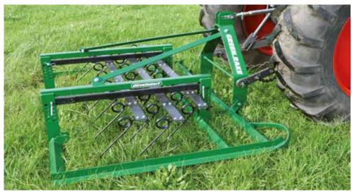
The municipal rake *GREEN.RAKE* mini stands out with its compact size of 1.50 m or 2.00 m. The *GREEN.RAKE* mini is ideal for use in municipal areas or in fruit-growing and viticulture.
