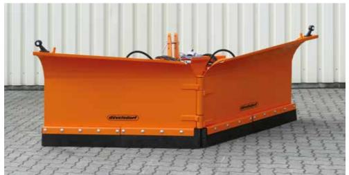
The düvelsdorf snow plough consists of two centrally mounted blade wings, which are individually hydraulically adjustable. Due to the flexible adjustment options of left, right, straight and as a plough, the snow blade is ideal for use in various areas such as streets, squares and farmyards.
