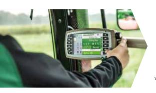
In addition to the use of a smartphone/tablet, operation (including parallel) can be executed via an ISOBUS terminal.
