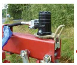
With this optional hydraulic drive (hydraulic drive limited by hoses), you control the log gripper's rotary movement easily and conveniently from the tractor seat.
