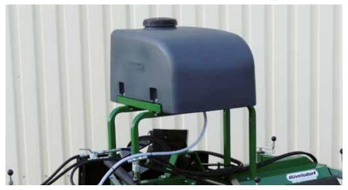
Spray equipment with 200 litre water storage tank
