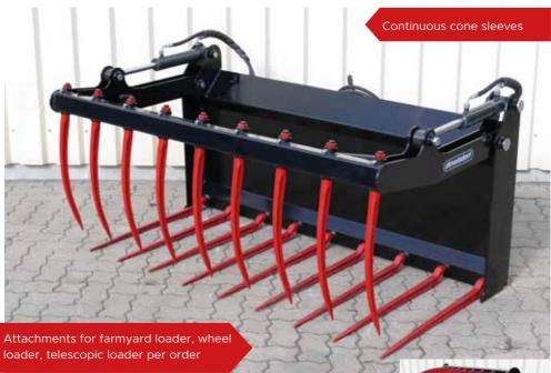
Practical manure and silage fork with hydraulic gripper. With two double-acting hydraulic cylinders, the tongs grip powerfully. This ensures that the goods to be transported remain safely on the fork. All tines are replaceable.
