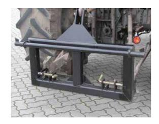
All front devices with quickexchange mounting (EURO standard) can be attached to the rear or front hydraulics of the tractor with the aid of the 3-point adapter.
