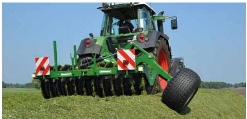
The silage roller, with its high tare weight and large drum, offers very good silage compaction with good rolling characteristics. The drum's twelve fins are used for deep compaction. When working in silage walls, the four rolling elements on the frame prevent damage to the silage roller and walls. By using the optional edge wheel (which can be retrofitted to any silage roller), the side/edge of the silage can be additionally compacted.
